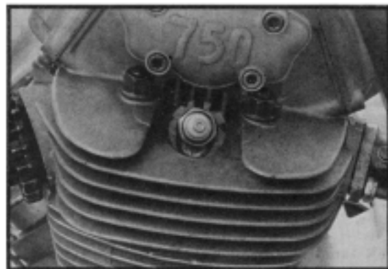
Heads were completely filled and re-shaped and spark plugs re-positioned higher in the combustion chamber after extensive flow-testing.
